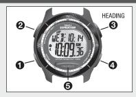
Press ① to cycle through time/date, chronograph, countdown timer, alarm. Compass function available in all modes except alarm by pressing ③ (HEADING).
